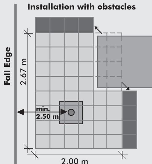
By moving the individual grid elements around, rising building elements or ventilation shafts, drains etc. can be embedded. Please note that the anchor point must not be positioned in either of the two outside grid rows. In addition, the Anchor Point must be placed in the centre of a grid element (0.33 × 0.33 m). In the stress direction, at least 20 grid elements must be behind the Anchor Point. We recommend having ZinCo plan and inspect such non-standard installation situations.
