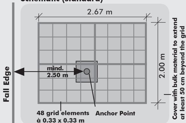
Schematic of a standard installation of the centred Anchor Point with the four pre-assembled grids (à 1.00 × 1.33 m).
