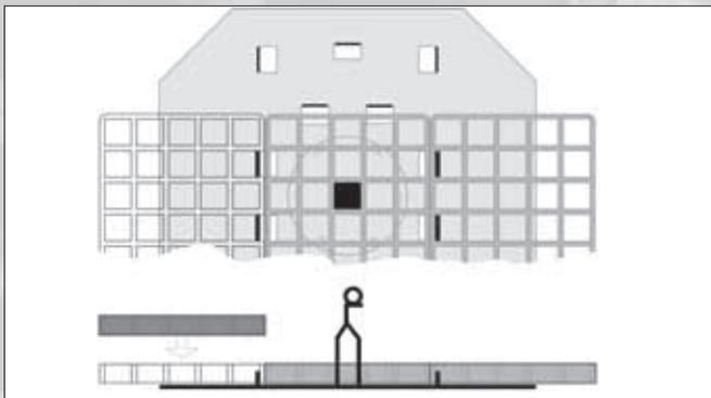
3. The grid must fully cover the base plate and the vertical locking tabs must engage the adjacent elements
